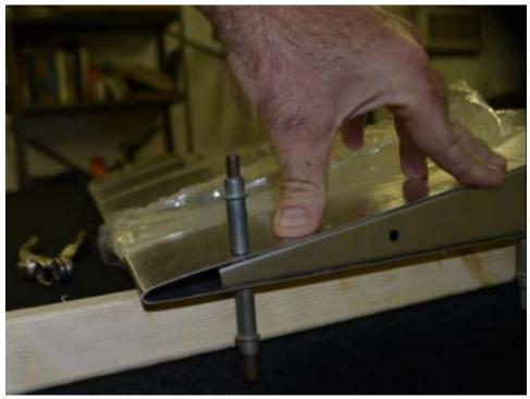
d. Move to the forward hole and drill pressing down firmly when drilling (see photo below)
