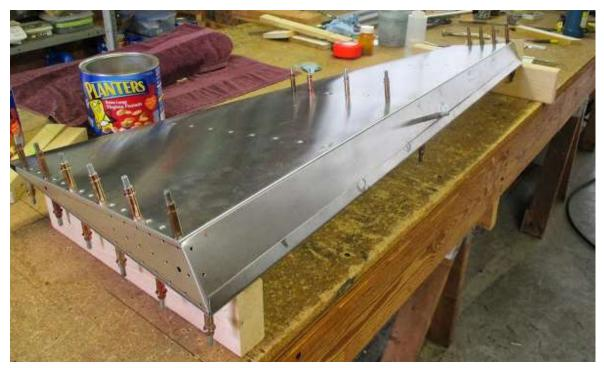
9. Align hinge on rudder per plans. Drill/ cleco #40 hinge using care so it and leading edge of rudder is straight.
