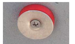
Inset, the isolator used for the automatic connection of the fuel sender unit in the wing. It's created by the 3D "printer."
